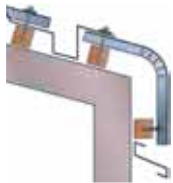
SYMMETRIC ROOF/WALL JOINT
